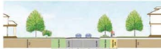
High Cross Road north of US150: 2-lane cross section with shoulders
