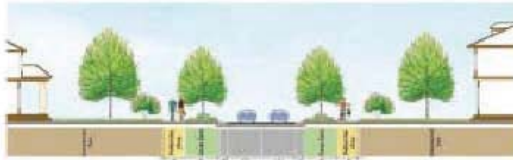
High Cross Road north of US150: 2-lane cross section with curb & gutter
