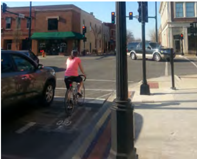
Figure 202 Bike-Activated Stoplight pavement marking on Race Street at Main Street
