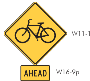
Figure 195 MUTCD Bicycle Warning Signage in advance of an intersection, without distance information (Signs W11-1 & W16-9P)
