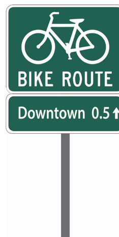
Figure 45 Bike Route sign with wayfinding signage that consists of destination, distance (in miles), and direction
