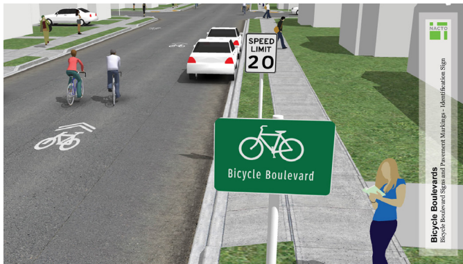
Figure 54 Bike Boulevard signs and pavement markings (Credit: NACTO Urban Bikeway Design Guide)
